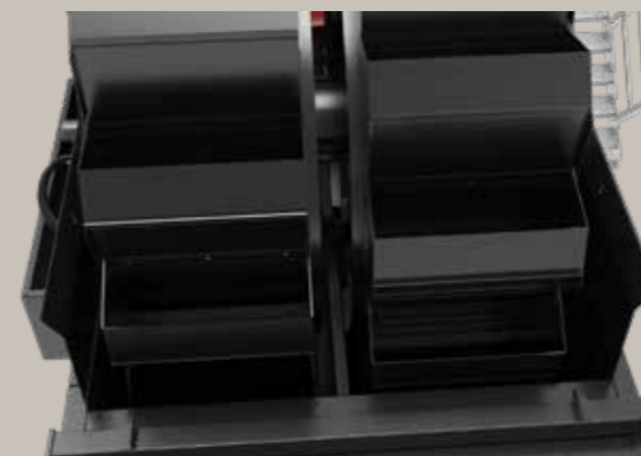
Anti-turbulence inlets in bucket tank
