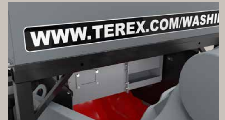
Movable chute to allocate fine material to the coarse product
