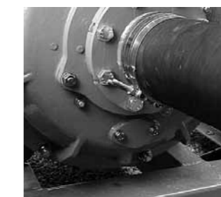
Pump drain for cold climate applications
